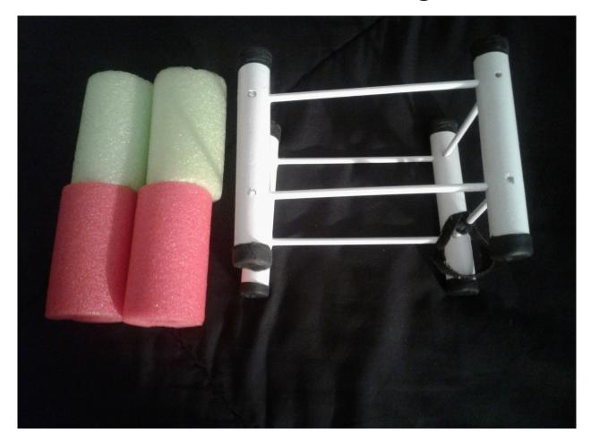
Above is a photo of an assembled and painted WISP Drone Carriage, that fits under any DJI Phantom 3 Standard Drone.
